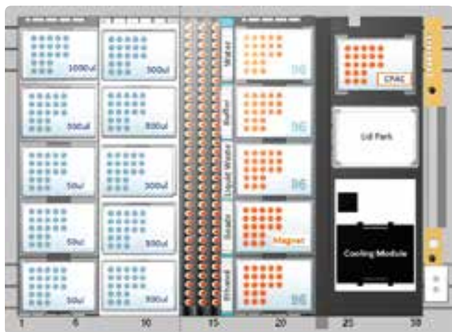
Figure 1: Deck Layout of the HAMILTON Starlet platform required for automated NEBNext DNA library preparation.
