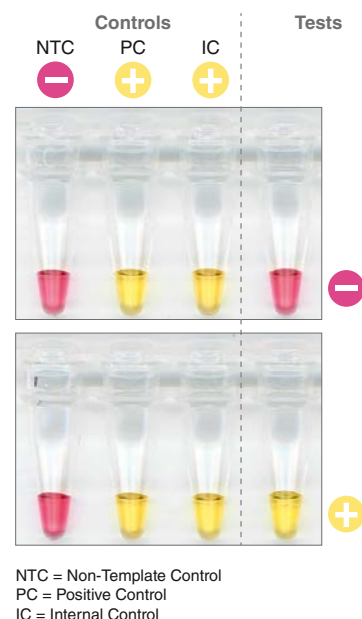
Figure 3: Rapid, simple, color-based detection of SARS-CoV-2 RNA
