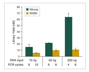
10, 50 and 200 ng Human NA12878 genomic DNA was sheared to 300 bp using the Covaris® S2 instrument and used as input into EM-seq and WGBS protocols. For WGBS, NEBNext Ultra II DNA was used for library construction, followed by the Zymo Research EZ DNA Methylation-Gold™ Kit for bisulfite conversion. For all input amounts, EM-seq library yields were higher, and fewer PCR cycles were required, suggesting greater DNA loss in the WGBS protocol. Error bars indicate standard deviation.
