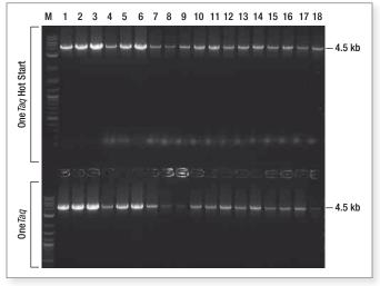
Reactions were set up according to the protocol and analyzed by agarose electrophoresis. Marker M is the 1 kb DNA Ladder (NEB #N3232)
